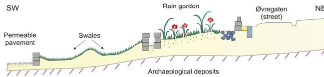
Section of the sustainable water management "treatment train", with rain garden, swales and permeable pavement. Drawing: Johannes de Beer, Geological Survey of Norway.
