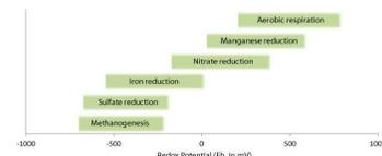
Overview over oxidation / reduction processes that control degradation of organic archaeological deposits, in relation to the Redox Potential (Eh) range in which they occur. At Bryggen, the Redox Potential is measured in conjunction with oxygen content to assess if the environment has become more stable. Graph: Michel Vorenhout, MvH Consult.
