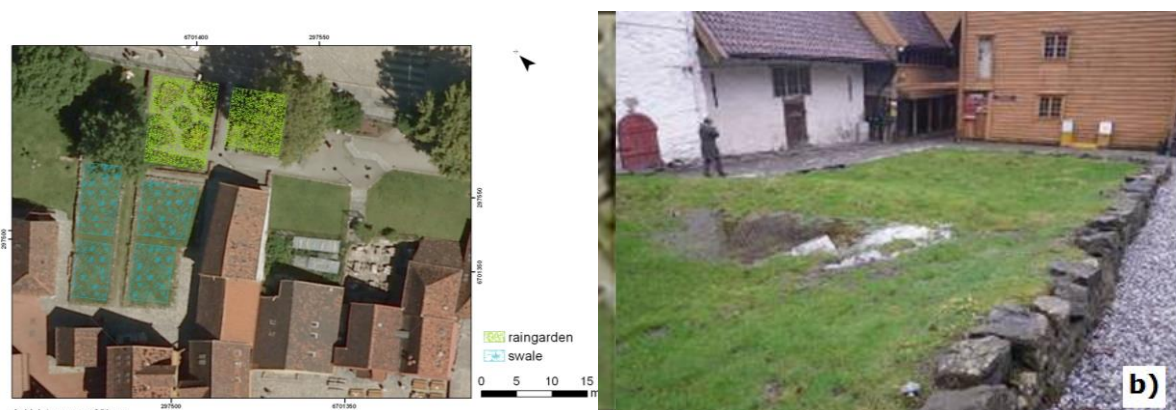
Figure 3: a) Site plan of Bryggen; b) Swales on Unesco world heritage site.
