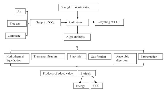
Figure 4. Schematic diagram of microalgae-mediated CO<sub>2</sub> bio capture and system integration (Modified from Zhou et al., 2017).
