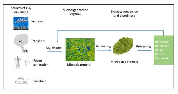
Figure 3. Schematic representation of microalgae cultivation, photosynthetic fixation of CO<sub>2</sub> into microalgae biomass and biomass processing.
