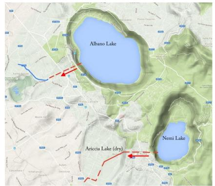
Fig. 4 – Lakes Albano, Nemi and Ariccia, the latter was dried up artificially in archaic times, probably during the 5<sup>th</sup> century AD. The red lines indicate the emissaries (the dashed lines indicate the underground sections).
