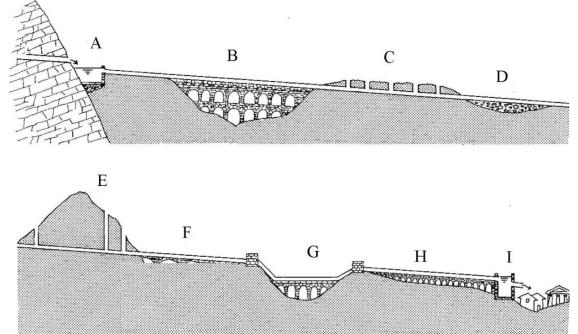
Fig. 3 – General sketch of the main constituents of a Roman aqueduct (partially redrawn after [3]).
