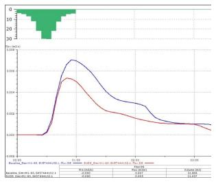
Figure 8 Model output showing reduced peak in sewer flow (in red)
