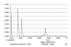
The installation of a data logger provides continuous water depth recording within the void space beneath one rain garden. The data obtained shows how the rain garden performs during and after rainfall. Variation in rain garden performance will be monitored over time.
