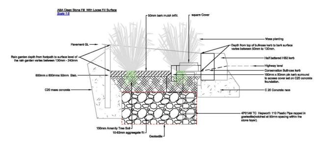
Figure 3 Section Drawing of the first rain garden design
